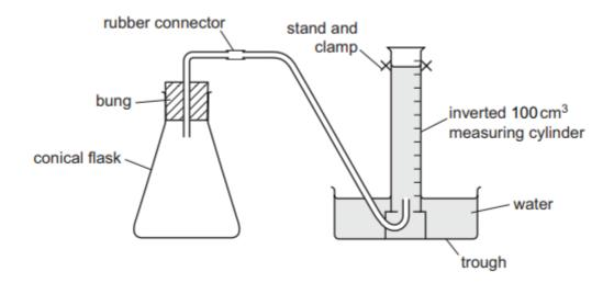
The hydrogen gas is collected in the measuring cylinder and its volume can be measured.
